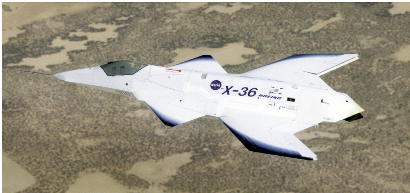
Figure 7: Image of X-36: "The X-36 Tailless Fighter Agility Research Aircraft, a 28% scale test aircraft, in flight, now part of the exhibit at the National Museum of the USAF in Dayton, Ohio"
